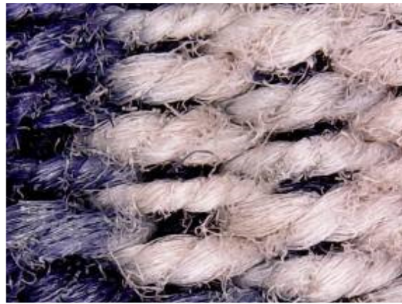
A microscopic detail of double-ply machine-made thread used in all ikated areas.
