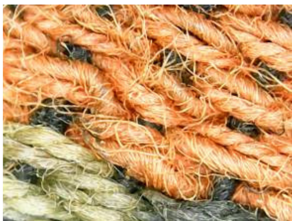
Hand-spun yarn and double-ply machine-made thread running in parallel, the latter in the white stripes.
