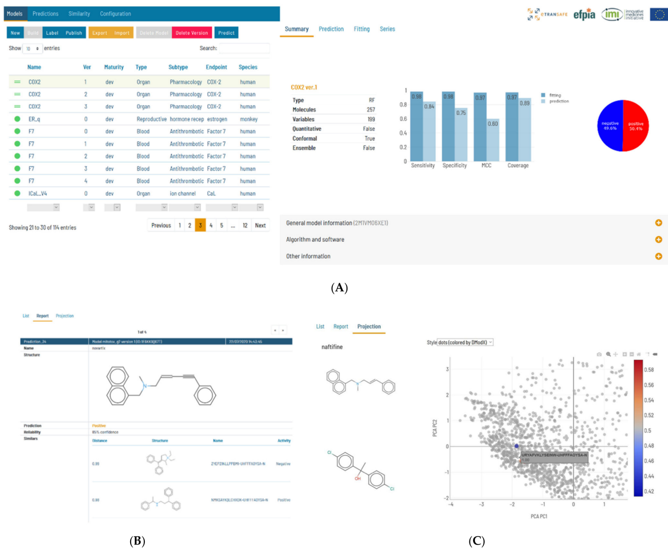
Figure 8. (A) Snapshot of the Flame graphical user interface showing on the left-hand side the model list and on the right-hand side information on the selected model, in this case a classifier. The selected tab presents an initial overview of the model quality and the proportion of positive and negative values. (B) A view of the prediction result that shows the compound structure, the prediction result and the associated confidence. The structure of the nearest compounds present in the training series is shown as a list. (C) In this view of the prediction results, the predicted compounds are represented in a PCA scores plot, together with the training series. The structures of the compounds are shown on mouse hover. The dots of the predicted compounds are coloured according to the distance to the model (DModX).
