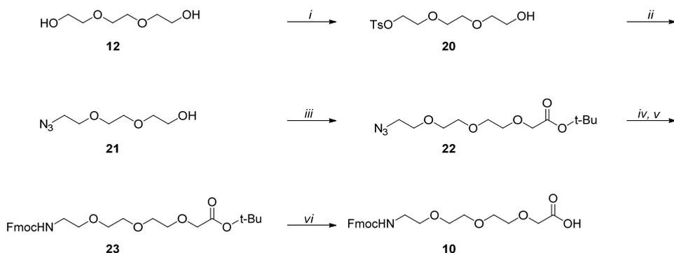
Scheme 3. Reagents and conditions: (i) TsCl, Et<sub>3</sub>N, DCM, 0 °C to rt, 17 hrs, 98% (ii) NaN<sub>3</sub>, DMF, 90 °C, 4 hrs, 82% (iii) KO<sup>t</sup>Bu, *tert*-butyl bromoacetate, <sup>t</sup>BuOH, 30 °C to 50 °C, 6 hrs, 80% (iv) PPh<sub>3</sub>, H<sub>2</sub>O, THF, 0 °C to rt, 41 hrs, 89% (v) Fmoc NHS ester, *N*-methylmorpholine, DCM, 0 °C, 6 hrs, 96% (vi) 85% wt% aq. H<sub>3</sub>PO<sub>4</sub>, toluene, 4 hrs, 98%.
