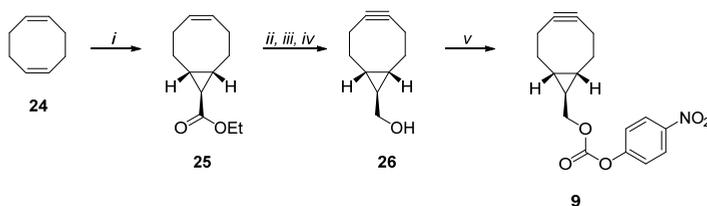
*Scheme 4.* Reagents and conditions: (i) ethyl diazoacetate, copper(II)acetylacetonate, EtOAc, reflux, 17 hrs, 44% (ii)  $\text{LiAlH}_4$ ,  $\text{Et}_2\text{O}$ , rt, 15 min. (iii)  $\text{Br}_2$ , DCM, 0 °C, 5 min. (iv)  $\text{KO}^t\text{Bu}$ , THF, reflux, 2 hrs, 56% over 3 steps (v) *p*-nitrophenyl chloroformate, pyridine, DCM, rt, 15 min, 69%.
