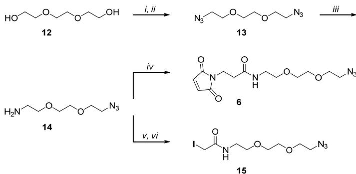
*Scheme 1.* Reagents and conditions: (i) TsCl, NaOH, DCM, 0 °C, 3 hrs, 91% (ii) NaN<sub>3</sub>, TBAI, DMF, 80 °C, 17 hrs, 91% (iii) PPh<sub>3</sub>, Et<sub>2</sub>O, THF, 1.0 M aq. HCl, rt, 24 hrs, 71% (iv) (a) 3-maleimidopropionic acid NHS ester, DIPEA, THF, rt, 4 hrs, 10% (b) 3-maleimidopropionic acid, 1-(3-dimethylaminopropyl)-3-ethylcarbodiimide hydrochloride, DIPEA, DCM, rt, 17 hrs, <5% (v) chloroacetyl chloride, Et<sub>3</sub>N, DCM, 0 °C, 2 hrs, 68% (vi) NaI, acetone, rt, 48 hrs, 84%.
