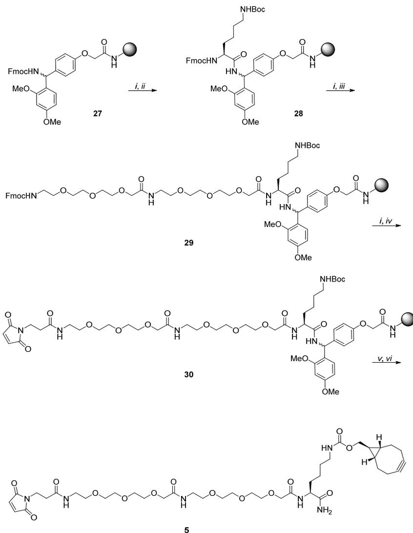
Scheme 5. Reagents and conditions: (i) piperidine, DMF, rt, 20 min (ii) Fmoc-Lys(Boc)-OH, HCTU, DIPEA, DMF, rt, 1 hr (iii) **10**, HCTU, DIPEA, DMF, rt, 1 hr (iv) 3-maleimidopropionic acid NHS ester, DIPEA, DMF, rt, 4 hrs (v) TFA – H<sub>2</sub>O – TIPS (190:5:5), rt, 3 hrs (vi) **9**, DIPEA, DMF, rt, 4 hrs, 25%.
