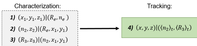
Figure 5.7: Schematic summary of the fitting steps performed to obtain the 3D position of a particle from the measured hologram analysis. The position in time is fitted in four steps: the first three are characterization steps, in which we find the approximate 3D position (fitting step 1) as well as appropriate guesses for the refractive index n (fitting step 2) and radius R (fitting step 3). In the fourth step, we use these positions and the average n and R values to determine the 3D position accurately (fitting step 4).
