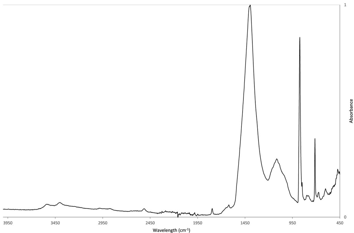
Fig. 6. FTIR spectrum of limestone from Abri Pataud.
