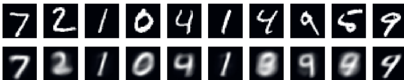
Figure 6.9: Reconstruction of MNIST data by a sparse autoencoder. The results are a bit less sharp than that of the ordinary autoencoder.
