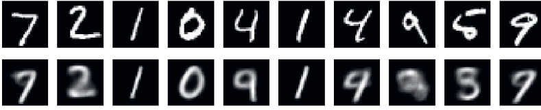
Figure 6.3: Reconstruction of MNIST data by a variational autoencoder. Top: the input, images with single hand-drawn digits. Bottom: the output, the images reconstructed by the autoencoder. During the training process the network weights are adjusted precisely so that the reconstruction loss between the output and the input is minimized. The variational autoencoder minimizes at the same time also the KL-divergence between the latent variables and a prior.
