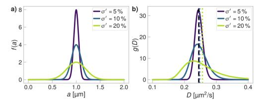
Figure 5.10: The collective diffusion constant depends on size polydispersity. a) Three hypothetical particle size distribution with an average particle radius of 1  $\mu$ m and relative polydispersities of 5 %, 10 % and 20 %. b) The distributions in diffusion constant corresponding to the three particle size distribution in panel a. The average diffusion constants are indicated by dashed lines. The average diffusion constant of a monodisperse sample is indicated by a black dashed line.
