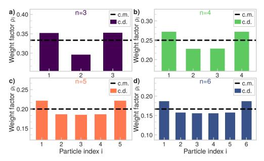
Figure 6.7: Center of diffusion (c.d.) versus center of mass (c.m.): weight factors. Weight factors  $\rho$  for the c.m. and the c.d., for **a**) trimer (n=3) **b**) tetramer (n=4) **c**) pentamer (n=5) **d**) hexamer (n=6) chains. For the c.d., more weight is accorded to the outer particles compared to the inner particles of the chain. However, differences between the c.m. and the c.d. are small for all chain lengths.
