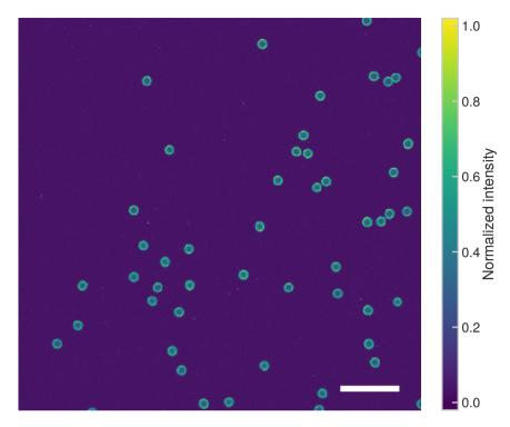
Figure 3.7: **Overview picture showing the homogeneity of the lipid bilayer** for CSLBs containing 1 mol % DOPE-PEG(2000). The scale bar is 15 μm.
