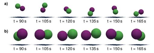
Figure 2.6: **Dumbbell orientation and height as function of time. a)** Schematics based on the experimentally tracked positions of a 2.2  $\mu$ m dumbbell at random times, showing out of plane rotations in addition to height variations. **b)** Schematics based on the experimentally tracked positions of a 4.2  $\mu$ m dumbbell at the same times as in panel a, showing significantly fewer out of plane rotations compared to the smaller dumbbell of panel a.
