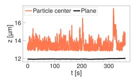
Figure 2.3: **Sphere-wall gap height.** The z positions of a spherical particle diffusing above a wall, as well as that of the plane (directly below the particle) obtained from the positions of three spheres fixed on the wall, are plotted in time. Using the plane z position, the gap height  $h_g$  between the diffusive particle and wall is determined.
