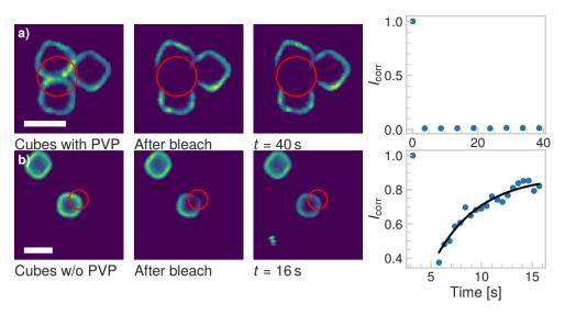
Figure 3.4: **Effect of PVP on CSLB formation.** FRAP experiment on a group of three cubes with **a)** and without **b)** PVP. Only the sample without PVP shows recovery of the signal in the bleached area. Scale bars are  $2 \, \mu m$ .
