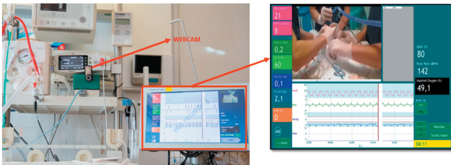
Figure 1. Recording equipment. Video is recorded by a webcam, capturing the neonate and providers' hands. Vital parameters include positive end-expiratory pressure and peak inspiratory pressure (pink), flow and respiratory rate (green), expired tidal volume (blue) and mask leak (orange), oxygenation, heart rate, and fraction of inspired oxygen. All measurements are digitized and recorded at 200 Hz using the Bicore II (Cardinal Healthcare, Yorba Linda, CA, USA) physiological recording system with Polybench software (Advanced Life Diagnostics, Weener, Germany).
