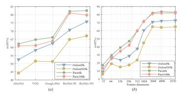
Fig. 11: (a) The effectiveness of different DCNNs on 4 datasets. All models are fine-tuned by the same loss function. The results are tested on the convolutional features with default dimension; (b) The impact of feature dimension on retrieval performance. These features are extracted by using ResNet-50.
