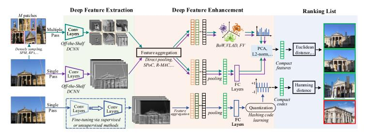
Fig. 1: In deep image retrieval, feature embedding and aggregation methods are used to enhance the discrimination of deep features. Similarity is measured on these enhanced features using Euclidean or Hamming distances.
