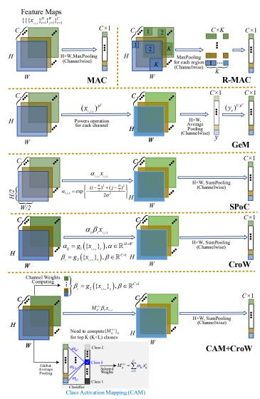
Fig. 4: Representative methods in single feedforward frameworks, focusing on convolutional feature maps x with size  $H \times W \times C$ : MAC [47], R-MAC [27], GeM pooling [41], SPoC with the Gaussian weighting scheme [7], CroW [10], and CAM+CroW [28]. Note that  $g_1(\cdot)$  and  $g_2(\cdot)$  represent spatialwise and channel-wise weighting functions, respectively.
