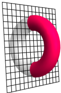
Figure 2.11: Schematic of the poloidal plane of a toroidal object (shown as a torus) as used in this work.
