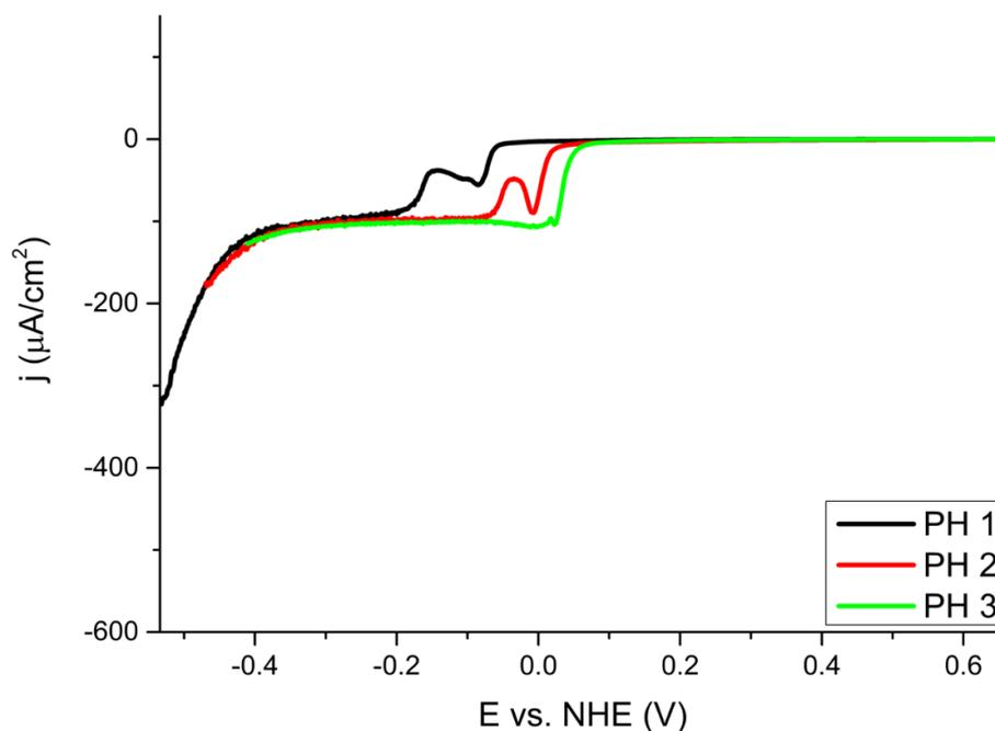
**Figure 13.** Linear sweep voltammograms of tin deposition from sulfuric acid at different pHs (1, 2, 3) on a gold rotating disc electrode. Concentration of solution:  $\text{Sn}^{2+}$  0.6 mM, scan rate  $2 \text{ mV s}^{-1}$ ; rotation rate 900 rpm.
