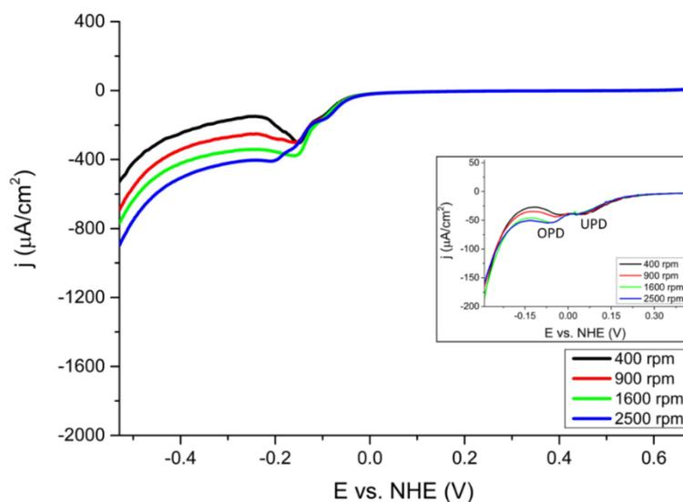
**Figure 11.** Linear sweep voltammograms of tin deposition from methanesulfonic acid on a gold rotating disc electrode. Concentration of solution  $\text{Sn}^{2+}$  0.6 mM, 0.1 M  $\text{CH}_3\text{SO}_3\text{H}$ . Scan rate  $30 \text{ mV s}^{-1}$ ; rotation rate 400, 900, 1600 and 2500 rpm. Inset tin deposition from 0.1 mM  $\text{Sn}(\text{CH}_3\text{SO}_3)_2$ , 0.1M  $\text{CH}_3\text{SO}_3\text{H}$
