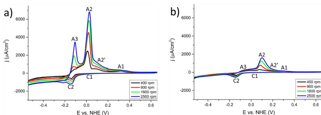
**Figure 6.** Cyclic voltammograms of tin deposition from sulfuric and methanesulfonic acid at a rotating gold disc electrode. Concentration of solution  $\text{Sn}^{2+}$  0.6 mM a) 0.1 M  $\text{H}_2\text{SO}_4$  b) 0.1 M  $\text{CH}_3\text{SO}_3\text{H}$ . Scan rate  $30 \text{ mV s}^{-1}$ ; rotation rate indicated in the figures
