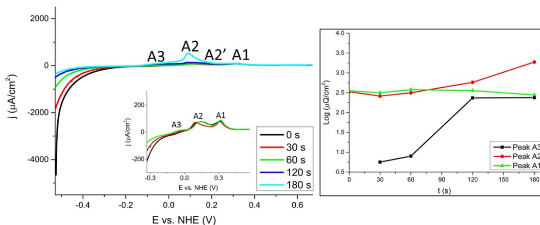
**Figure 8.** Stripping voltammograms of tin deposition from methanesulfonic acid. Concentration of solution  $\text{Sn}^{2+}$  0.1 mM.  $30 \text{ mV s}^{-1}$  and 900 rpm from 0.1 M  $\text{CH}_3\text{SO}_3\text{H}$ . Potential was kept at -0.529V during different periods of time, -0.529 V was chosen as starting potential.
