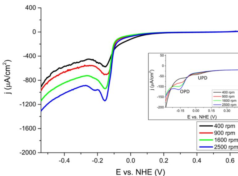
**Figure 10.** Linear sweep voltammograms of tin deposition from sulfuric acid on a gold rotating disc electrode. Concentration of solution  $\text{Sn}^{2+}$  0.6 mM. Scan rate  $30 \text{ mV s}^{-1}$ ; rotation rate 400, 900, 1600 and 2500 rpm inset, tin deposition from 0.1 mM  $\text{SnSO}_4$ , 0.1 M  $\text{H}_2\text{SO}_4$ .
