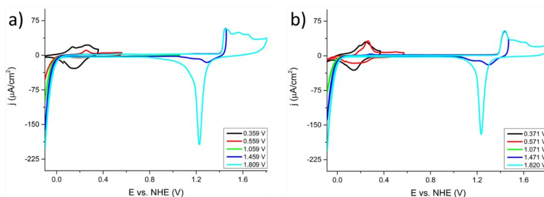
**Figure 5.** Voltammetric desorption of tin adspecies in the test electrolyte. Tin was adsorbed from a deaerated tin solution of 1 mM  $\text{SnSO}_4$  (A) and  $\text{Sn}(\text{CH}_3\text{SO}_3)_2$  (B) and then transferred to a test solution a) 0.1M  $\text{H}_2\text{SO}_4$  and b) 0.1 M  $\text{CH}_3\text{SO}_3\text{H}$ .
