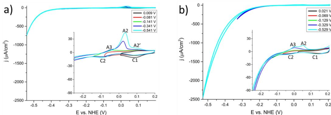
**Figure 4.** Cyclic voltammograms of a polycrystalline gold electrode, different switching cathodic potentials at  $10 \text{ mV s}^{-1}$ . a)  $0.1 \text{ M H}_2\text{SO}_4 - 0.1 \text{ mM SnSO}_4$  b)  $0.1 \text{ M CH}_3\text{SO}_3\text{H} - 0.1 \text{ mM Sn (CH}_3\text{SO}_3)_2$
