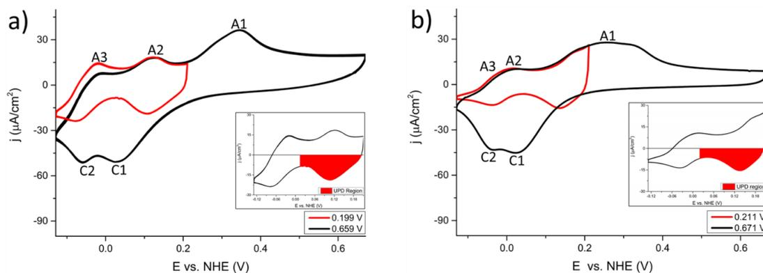
**Figure 2.** Cyclic voltammograms of tin electrodeposition on a polycrystalline gold electrode for different switching anodic potentials at 30 mV s<sup>-1</sup>. a) 0.1 M H<sub>2</sub>SO<sub>4</sub>, 0.1 M SnSO<sub>4</sub> b) 0.1 M CH<sub>3</sub>SO<sub>3</sub>H, 0.1 M Sn(CH<sub>3</sub>SO<sub>3</sub>)<sub>2</sub>.
