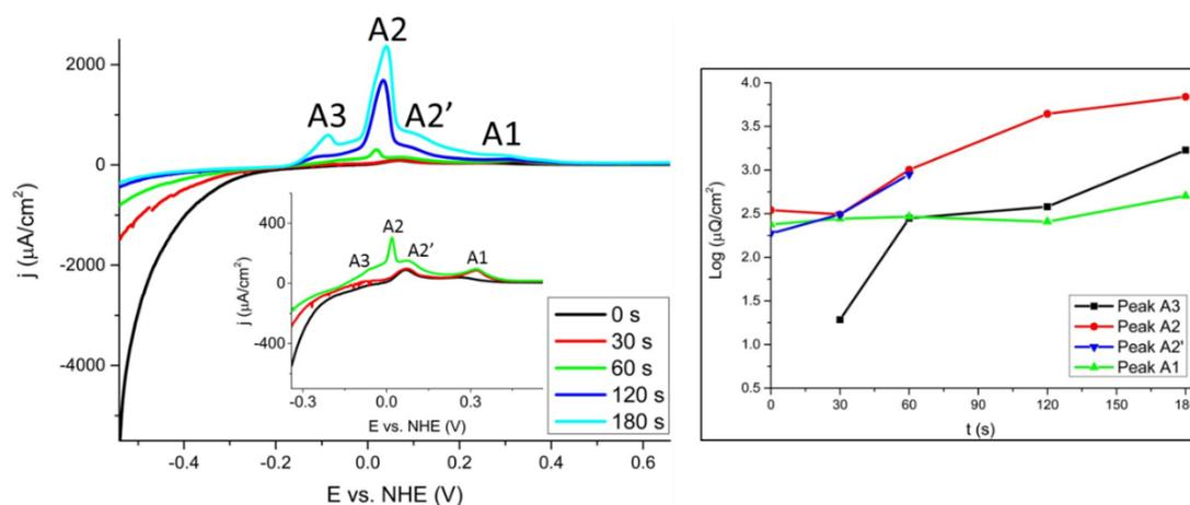
**Figure 7.** Stripping voltammograms of tin deposition from sulfuric acid. Concentration of solution  $\text{Sn}^{2+}$  0.1 mM.  $30 \text{ mV s}^{-1}$  and 900 rpm from 0.1 M  $\text{H}_2\text{SO}_4$ . Potential was kept at  $-0.541 \text{ V}$  during different periods of time,  $-0.541 \text{ V}$  was chosen as starting potential.
