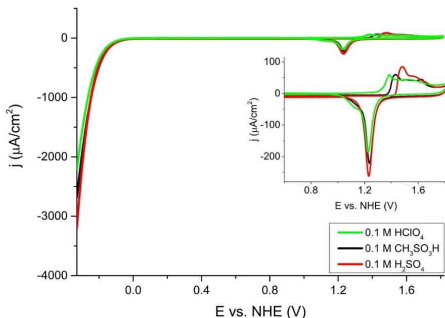
**Figure 1.** Cyclic voltammograms of a polycrystalline gold disc electrode, 0.1 M H<sub>2</sub>SO<sub>4</sub> (red line) and 0.1 M CH<sub>3</sub>SO<sub>3</sub>H (black line) and 0.1 M HClO<sub>4</sub> (green line) recorded between -0.34 to 1.81 V in SA and -0.33 to 1.82 V vs. NHE in MSA at 50 mV s<sup>-1</sup>.
