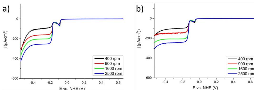
**Figure 12.** Linear sweep voltammograms of tin deposition from sulfuric and methanesulfonic acid on a gold rotating disc electrode. Concentration of solution a)  $\text{Sn}^{2+}$  0.6 mM, 0.1 M  $\text{H}_2\text{SO}_4$  and b) 0.1M  $\text{CH}_3\text{SO}_3\text{H}$ . Scan rate  $2 \text{ mV s}^{-1}$ ; different rotation rates.
