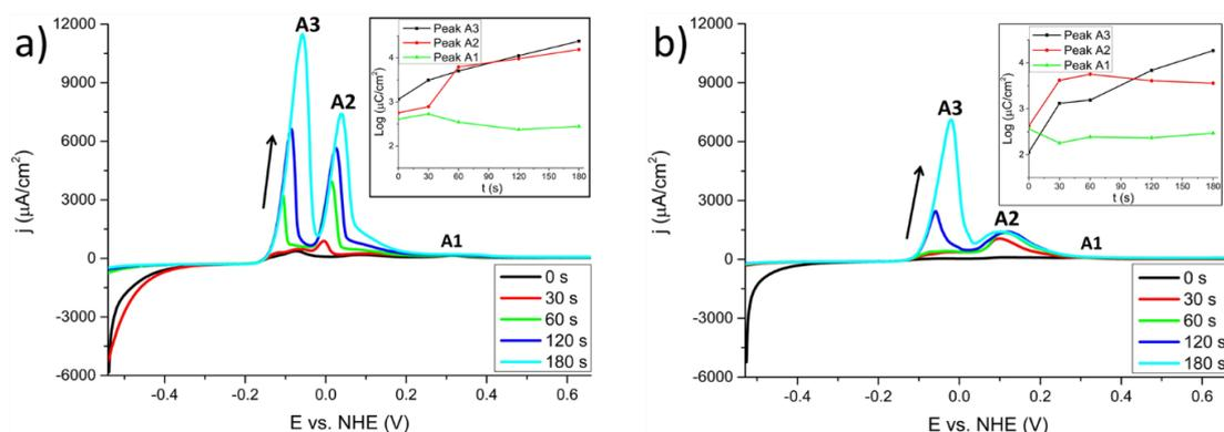
**Figure 9.** Stripping voltammograms of tin deposition from sulfuric and methanesulfonic acid. Concentration of solution  $\text{Sn}^{2+}$  0.6 mM.  $30 \text{ mV s}^{-1}$  and 900 rpm from 0.1 M  $\text{H}_2\text{SO}_4/\text{CH}_3\text{SO}_3\text{H}$ . Potential was kept at  $-0.541 \text{ V}$  (SA) and  $-0.529 \text{ V}$  (MSA) during different periods of time, previous potentials were chosen as starting potentials.
