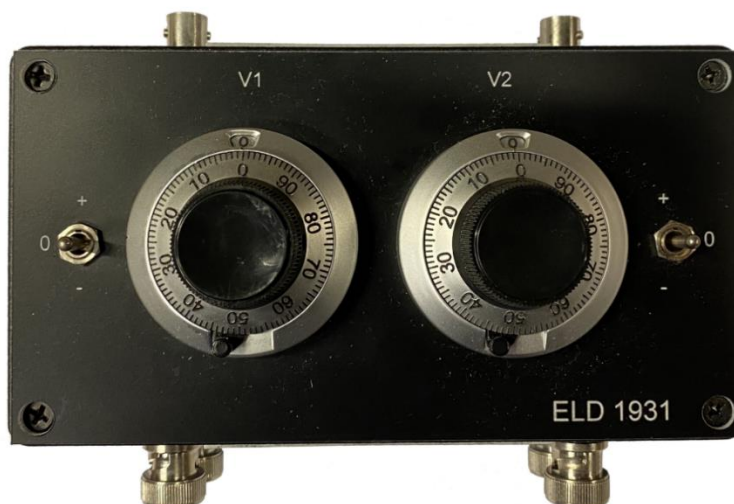
Figure 6.4: Home-made battery-fed power supply with two outputs and 0.5 mV resolution.
