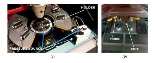
Figure 14: Measurement setup for strain gauge measurement.
