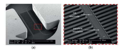
Figure 9: SEM image of the Cytostretch chip.
