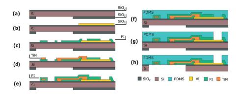
Figure 8: Process flow for the MEA module.
