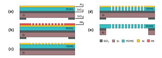
Figure 4: Process flow for the through-membrane micro-pore array.
