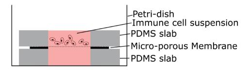
Figure 5: Schematic of setup for simple migration experiment.
