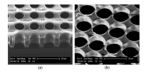
Figure 6: SEM images of microporous PDMS membranes.
