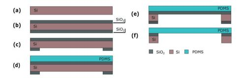
Figure 3: Process flow for the product platform.
