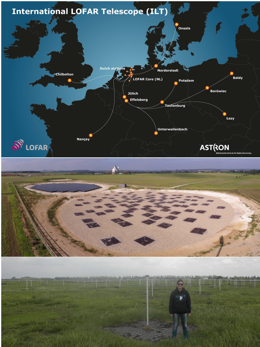
Figure 4: Top : The locations of LOFAR stations. The data in this thesis were taken before the stations in Poland were constructed, when the longest baseline was between Onsala and Nancay (1292km). Middle : The LOFAR-UK station at Chilbolton. The LBA antennas are in the foreground with the HBA antennas clustered together under a weather-protective covering behind the LBA. Bottom : Dipoles from an LBA station within the central core of LOFAR, with the author in the picture for scale.
