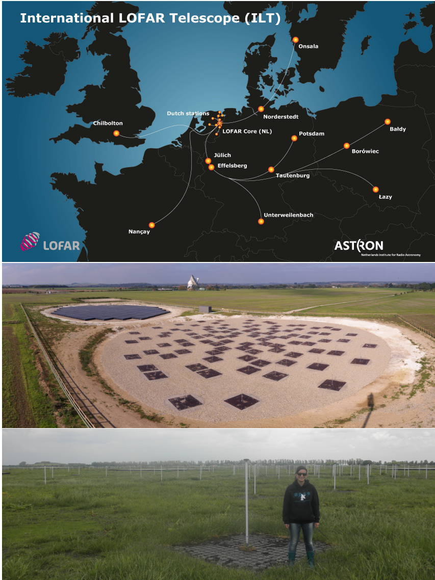
Figure 1.4: Top : The locations of LOFAR stations. The data in this thesis were taken before the stations in Poland were constructed, when the longest baseline was between Onsala and Nançay (1292km). Middle : The LOFAR-UK station at Chilbolton. The LBA antennas are in the foreground with the HBA antennas clustered together under a weather-protective covering behind the LBA. Bottom : Dipoles from an LBA station within the central core of LOFAR, with the author in the picture for scale.
