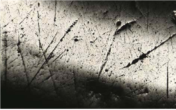
Figure 10. Wear traces seen on the sickle of Heiloo (orig. magnif. 100x).
