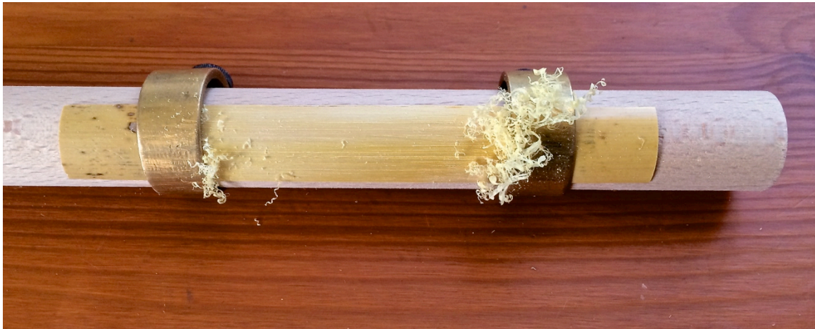
Figure 5.9. The first phase of bark removal in manual profiling
