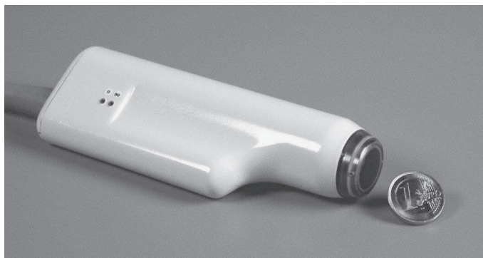
Figure 1.5: The fast rotating ultrasound (FRU) transducer
