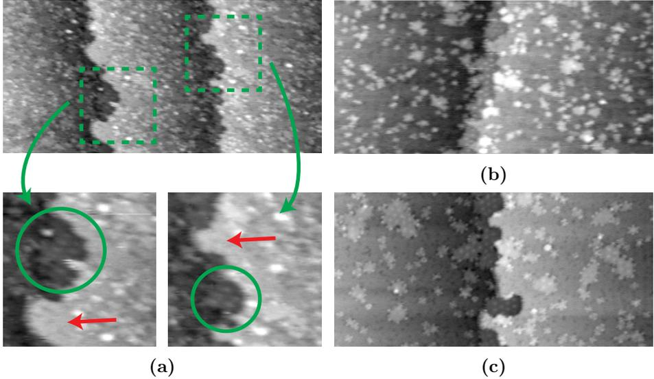
**Figure 6.6:** STM images of iridium recorded at (a) 967 K, (b) 995 K and (c) 1001 K, after exposure to 3 L of ethylene at room temperature. Two close-ups of the first image are presented to highlight the moiré patterns present (green circles) and to indicate areas without clusters at the iridium steps (red arrows). Image size  $125 \times 60 \text{ nm}^2$ , z-scale 0.26 nm, sample voltage 3.06 V for images (a) and (b), 2.73 V for image (c), tunnelling current 0.1 nA.
