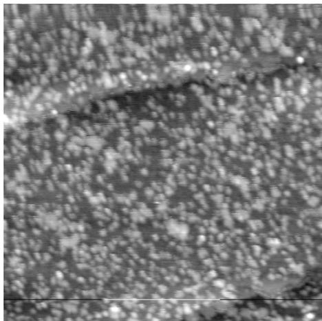
**Figure 6.4:** STM image of the iridium surface at a temperature of 865 K. Before heating, the surface had been exposed to 3 L of ethylene at room temperature. Image size  $125 \times 125 \text{ nm}^2$ , z-scale 0.35 nm, sample voltage 3.01 V, tunnelling current 0.1 nA.
