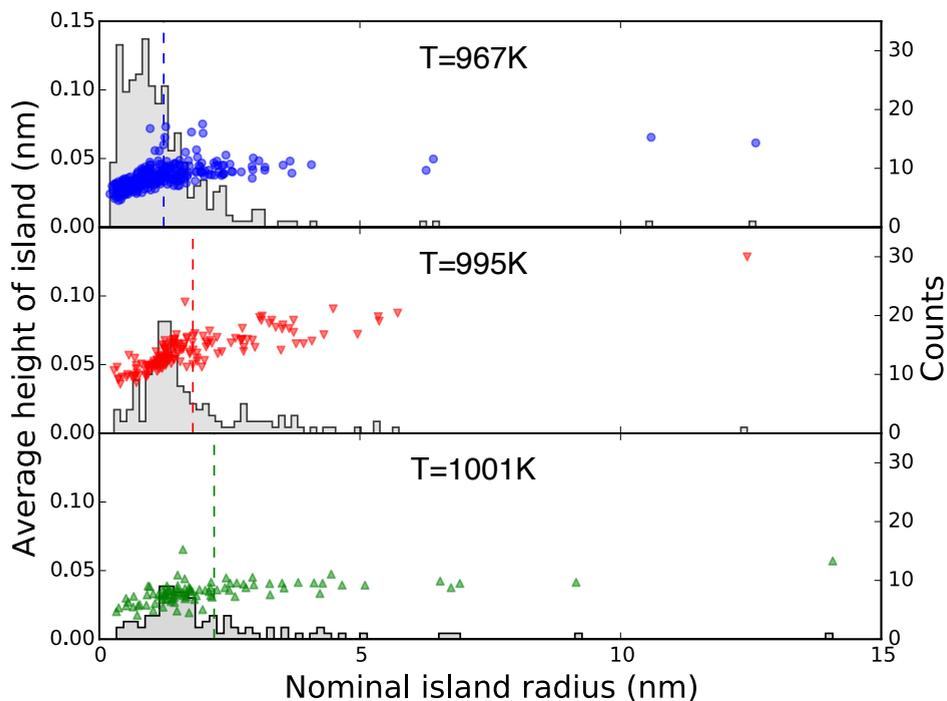
**Figure 6.8:** Observed distribution of nominal radii (histograms) and heights (symbols) of the islands in the STM images of Figure 6.6 at 967 K (top panel), 995 K (middle panel) and 1001 K (bottom panel). At each temperature, the dashed vertical line indicates the average island radius. The nominal radius of each island was obtained from the island’s area, assuming a perfectly circular shape. The island area was obtained by use of the island-extraction algorithm, described in Appendix D.
