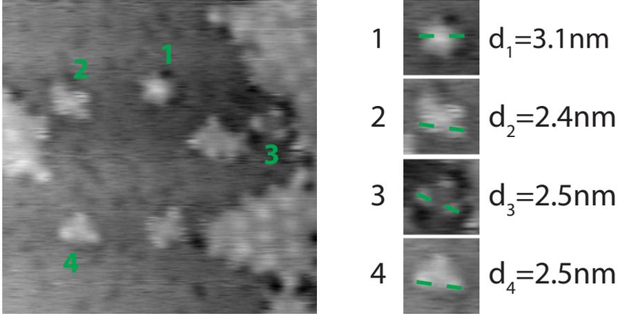
**Figure 6.9:** STM image of the iridium surface covered with graphene islands, recorded at 1014 K. Some islands are magnified to bring out the differences in orientation with respect to the substrate. Each orientation results in a specific apparent height of the graphene island and in a specific shape of the smallest stable unit of graphene. Image size  $30 \times 30 \text{ nm}^2$ , z-scale 0.13 nm, sample voltage 2.73 V, tunnelling current 0.1 nA.
