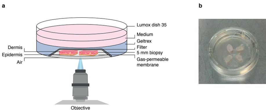
**Figure 1 | Setup of the *ex vivo* imaging system for skin biopsies.** **a**, Schematic overview of the *ex vivo* imaging setup. Note that a cross-section of the dish is shown to illustrate how the biopsies are placed on the gas-permeable membrane. In reality, the filter, Geltrex and medium enclose the biopsies. **b**, Representative image of healthy human skin biopsies mounted in the *ex vivo* imaging dish.
