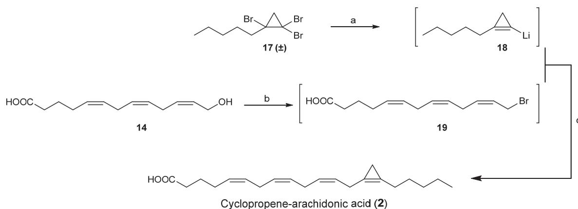
**Scheme 3 | Synthesis of cyclopropene-arachidonic acid (2).** Reagents and conditions: (a) *n*-BuLi, Et<sub>2</sub>O, -80 °C to rt, 25 min; (b) NBS, dimethyl sulfide, DCM, -25 °C to rt, 1 h; (c) HMPA, Et<sub>2</sub>O, 0 °C to rt, 15 min, 28%.
