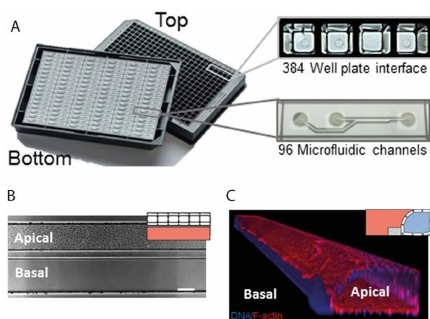
**Figure 3 | Microfluidic cell culture device: OrganoPlate.** (A) Photograph of bottom and top views of an OrganoPlate. The device consists of a 384 wells plate interface on top and 96 microfluidic chips integrated in the bottom. (B) Phase contrast image and (C) 3D reconstruction of a microvessel in the OrganoPlate [30].
