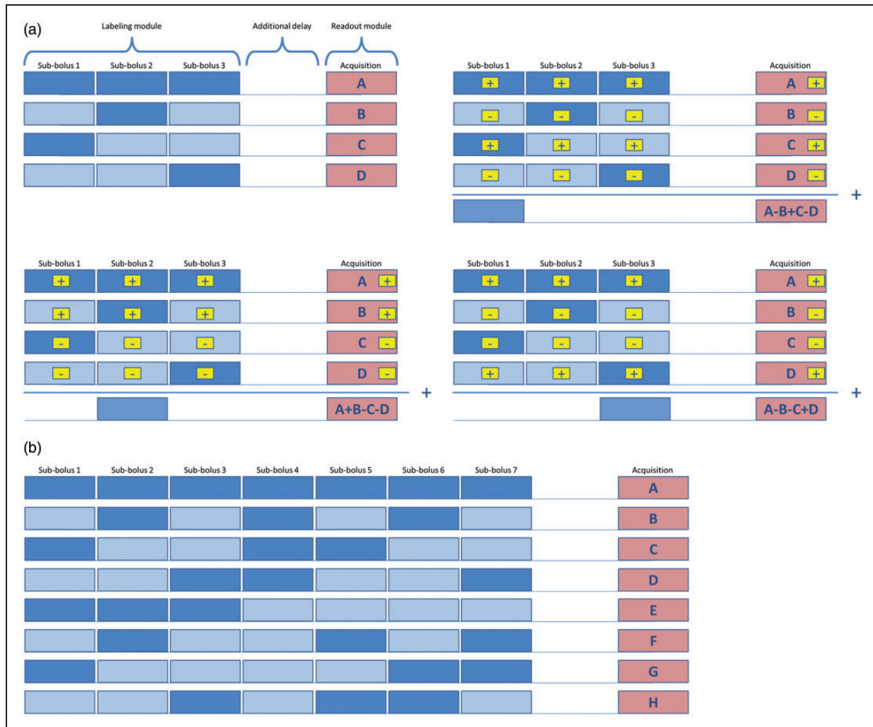
Figure 3. Schemes of Hadamard-4 (a) and Hadamard-8 (b) matrices for application in time-encoded ASL. For Hadamard-4 not only the encoding matrix is shown but also the three decoding options are presented that are employed for calculation of the individual sub-boli images. Summation (or subtraction) of images is indicated in the yellow boxes. Below the decoding matrix, the traditional (non time-encoded) ASL-scan is indicated, which will provide the same image with the same SNR as the decoded sub-bolus image (when similar total scan time is employed). Dark blue boxes indicate label condition of the pCASL-labelling; light blue boxes with dark blue wavy patterns indicate control condition of the pCASL-labelling; dark blue boxes with light blue wavy patterns indicate the result of the subtraction of control minus label condition, i.e. the ASL-signal. Pink boxes indicate imaging.
