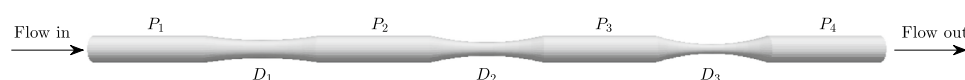
Fig. 1 An idealized three-dimensional axisymmetric coronary artery model with multiple coronary lesions in series. Diameters of stenosis (DOS) from left to right are: D_1 = 2 mm, D_2 = 1.5 mm and D_3 =
