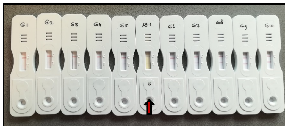
Fig. 2. Example of scoring a urine sample using the G-scores. The arrow indicates the cassette to be scored, which is placed in between the G-scores that resemble the intensity of the test line in order to select the best matching G-score.
