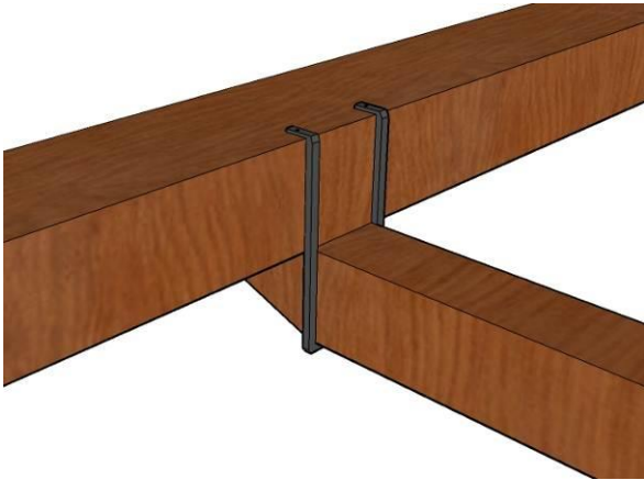
75 Hangbalk in strop
