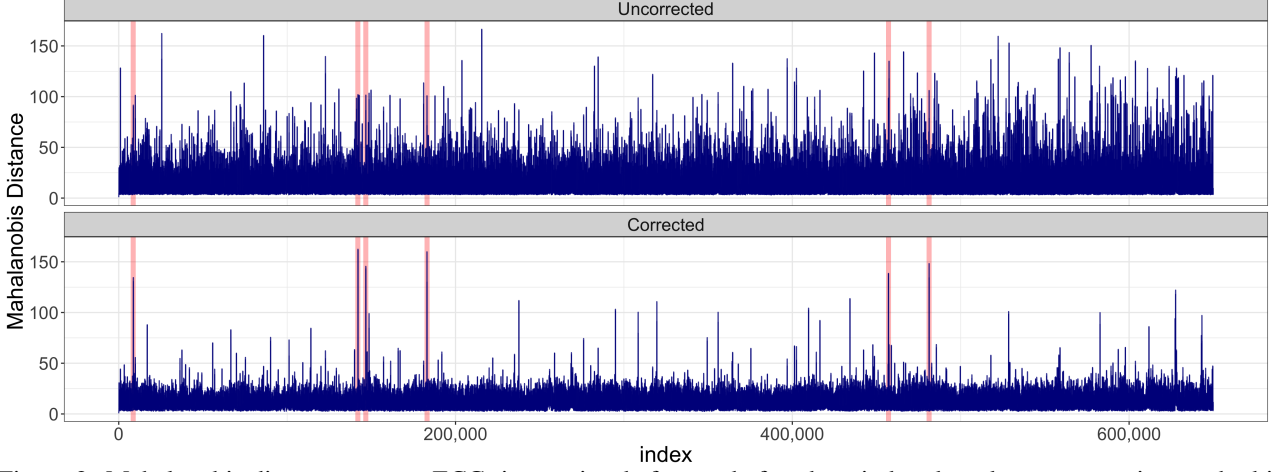
Figure 2: Mahalanobis distance over an ECG time series, before and after the window-based error correction method is applied.
