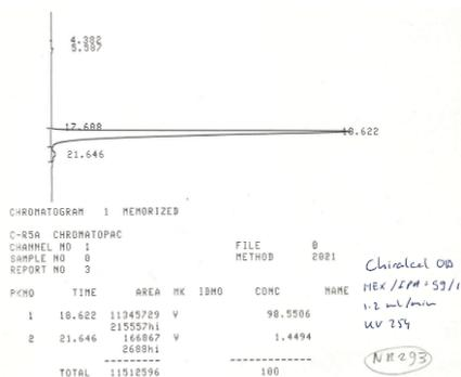
Figure 5. Analysis of ee of compound 16.
