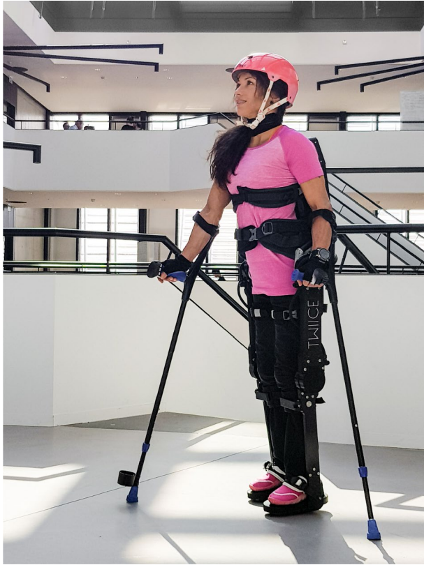
Fig. 2 Lightweight exoskeleton from TWICE (see http://twiice.ch/ , last accessed October 9, 2019)
