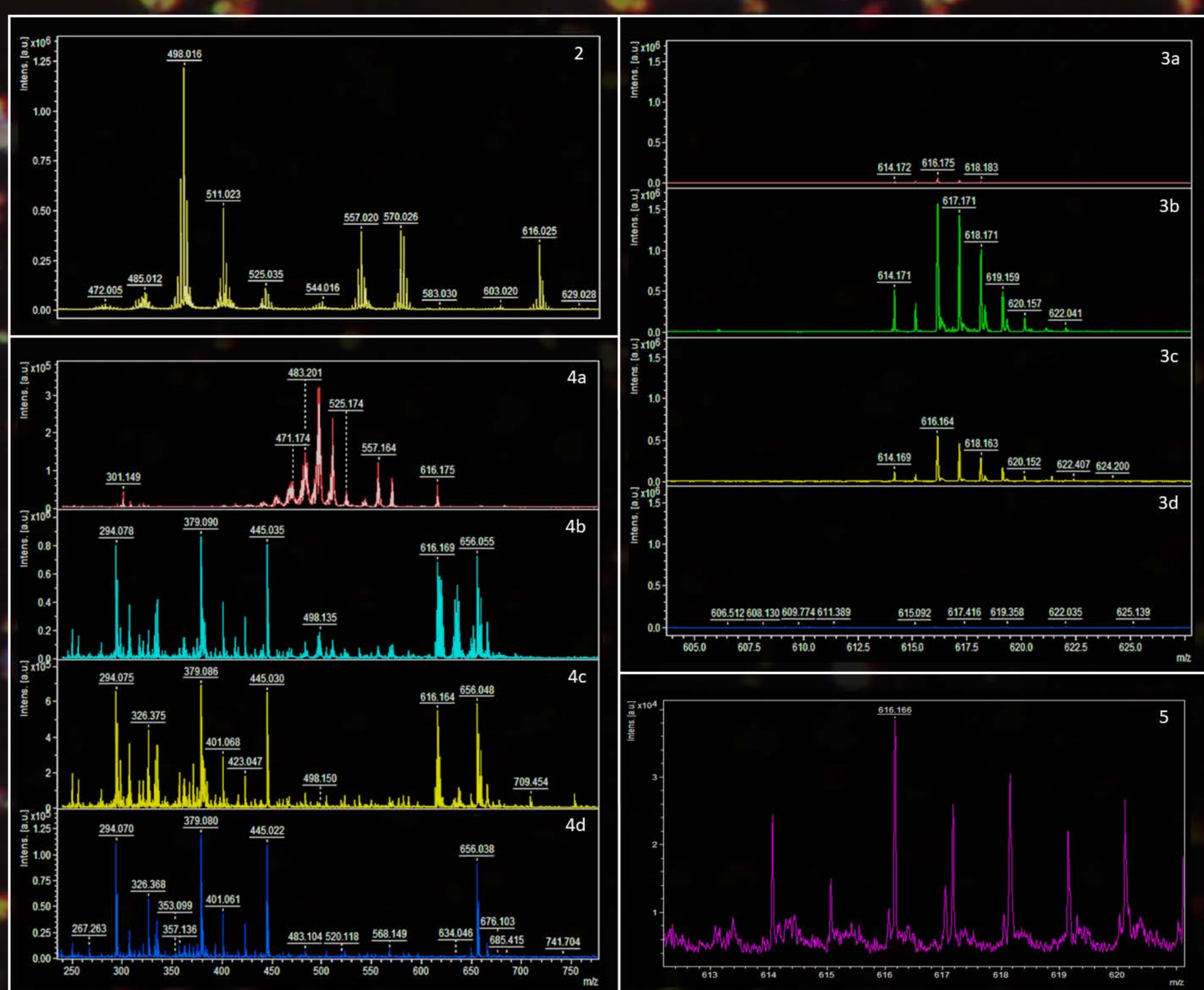
Fig. 2-5: Results initial analysis synthetic hemozoin. Fig. 2: Hemozoin MS signature (no matrix used). Fig. 3: 616 m/z region, a) hemozoin, no matrix, b) hemozoin in \text{CHCl}_3 with matrix, c) hemozoin in MQ with matrix, d) matrix (4-HCCA). Fig. 4: Suppression of fragment ions with matrix, a) hemozoin, no matrix, b) hemozoin in \text{CHCl}_3 with matrix, c) hemozoin in MQ with matrix, d) matrix (4-HCCA). Fig. 5: 616 m/z at 50 pg (signal to noise = 14).
