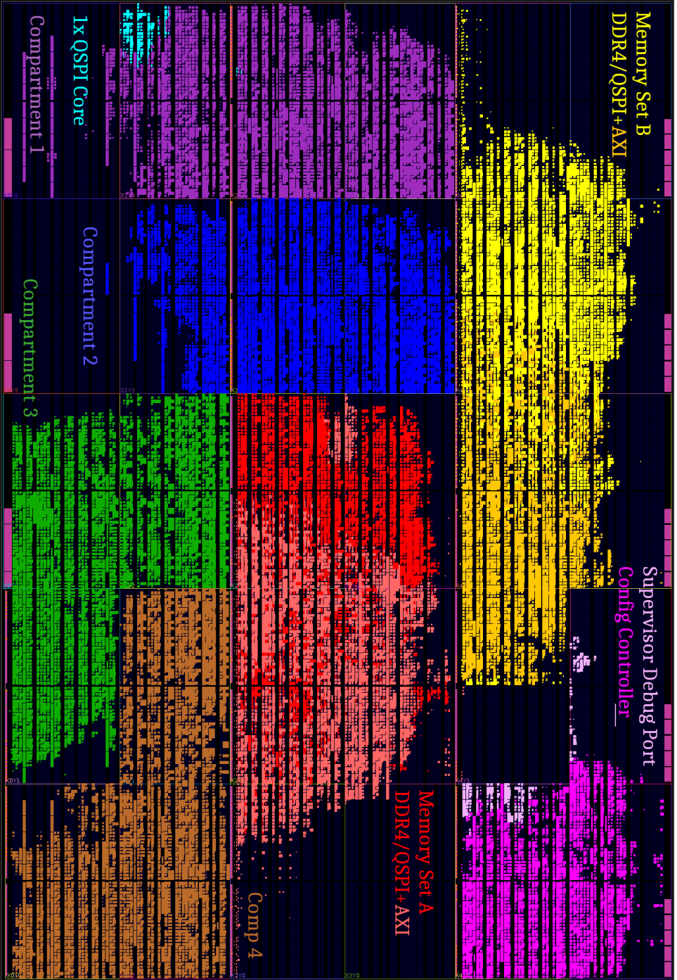
Figure 68: Logic placement of our proof-of-concept quad-core MPSoC for the upcoming XRT/C Kintex Ultrascale KU60 device-test board. A QSPI controller is highlighted in teal for size-comparison between an interface core and a compartment's total size.
