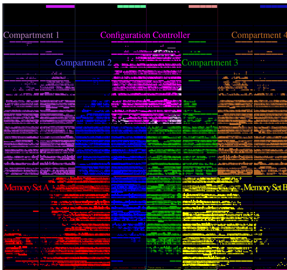
Figure 74: Logic placement of our proof-of-concept MPSoC on a Xilinx Kintex Ultrascale+ KU3P with 4 compartments (purple, blue, green, and brown), two shared memory controller sets (red & yellow) and static logic (pink). In contrast to the KU60 implementation, DDR controllers of this designs have reduced data width.
