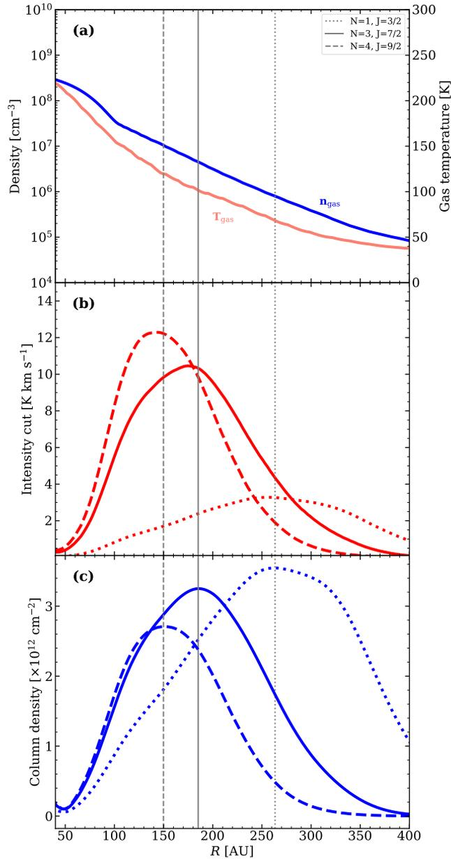
**Figure 5.19:** (a) Gas density and temperature along the CN high abundance layer (dotted-green line in Fig. 5.2a). (c) Column densities of CN molecules in the ( $N=1$ ,  $J=3/2$ ) (dotted), ( $N=3$ ,  $J=7/2$ ) (solid) and ( $N=5$ ,  $J=11/2$ ) (dashed) levels. (b) Intensities of the  $N=4-3$ ,  $N=3-2$  and  $N=1-0$  transitions, for comparison with panel (c). The vertical lines mark the location of the column density peaks of CN molecules in the three levels.
