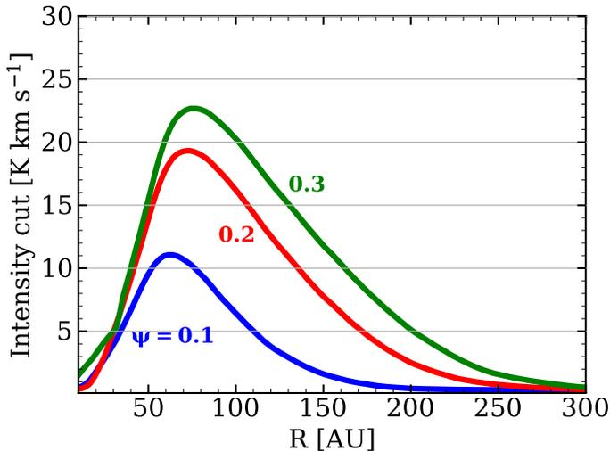
**Figure 5.10:** Different intensity radial profiles for  $\psi = 0.1, 0.2$  and  $0.3$  in a disk with  $M_{\text{disk}} = 10^{-2} M_{\odot}$  and  $h_c = 0.1$  rotating around a T Tauri star. The intensity of the CN emission increases in more flared disks and moves to slightly larger radii.
