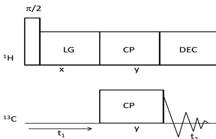
Figure 3. HETCOR  $^1\text{H}$ - $^{13}\text{C}$  LG-CP pulse sequence; this pulse sequence starts with  $90^\circ$  preparation pulse followed by the *Lee-Goldburg* decoupling during  $t_1$ . After that cross-polarization pulses are applied in mixing time on both  $^1\text{H}$  and  $^{13}\text{C}$ . During  $t_2$   $^{13}\text{C}$  FID is observed.
