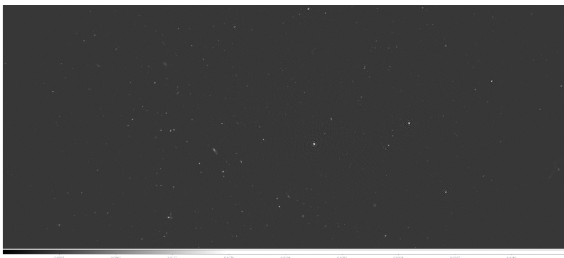
Figure 1.6: Full direction-dependent calibrated image of the L229587 data, done at a high resolution. This image shows a drastic reduction in imaging artifacts as well as a low image noise level. Some of the leftover artifacts are due to skipping the flux bootstrapping step, and using half the bandwidth
