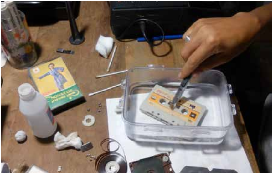
Figure 19. Acong placing a cassette into warm water to remove the damaged label, Kunci, Yogyakarta. Photo by the author.
