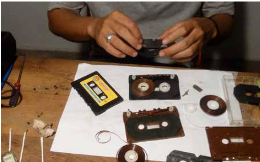
Figure 18. Along using two broken cassettes to repair another cassette, Kunci, Yogyakarta. Photo by the author.
