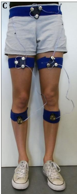
Marker set-up of the Optotrak system
