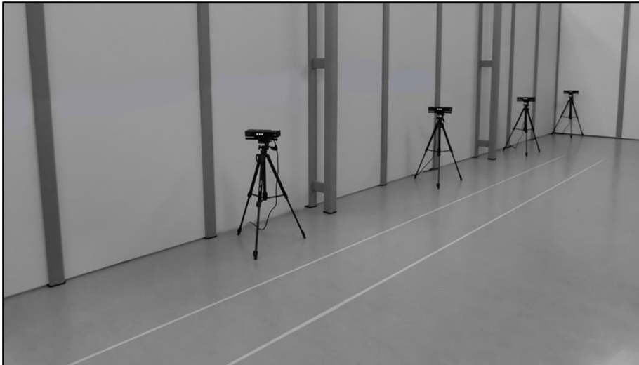
Figure 2.2 Overview of the multi-Kinect v2 set-up.
