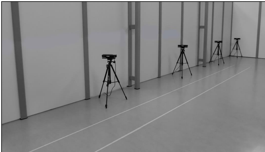
Figure 2.2 Overview of the multi-Kinect v2 set-up.
