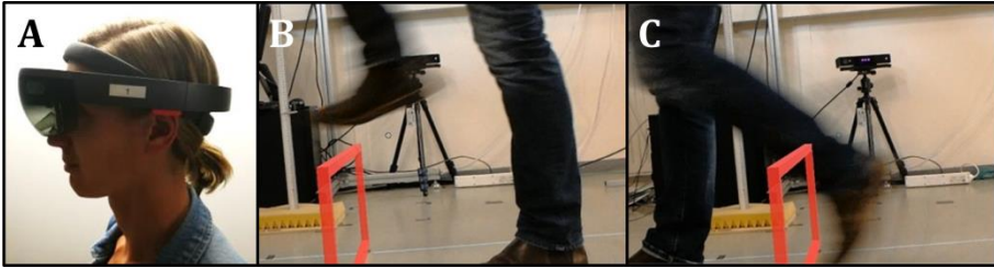
Figure 8.3 The HoloLens (A) and obstacle avoidance over a holographic obstacle presented with the HoloLens with the leading (B) and trailing (C) limb.
