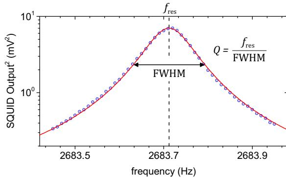
FIG. 2. Example of a frequency sweep measured at a tip-sample separation of  $3.4 \mu\text{m}$  at a temperature of  $25 \text{ mK}$ . The resonance frequency and quality factor are obtained by the fitting of the data to a Lorentzian (solid red line).
