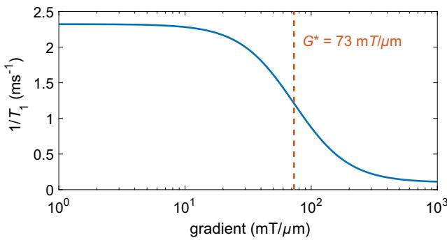
FIG. 5. Plot of the inverse of the  $T_1$  time calculated from Eq. (11), using  $G^* = 73 \text{ mT}/\mu\text{m}$ ,  $T_1^{\text{ff}} = 0.45 \text{ ms}$ , and  $T_1^* = 10 \text{ ms}$ .
