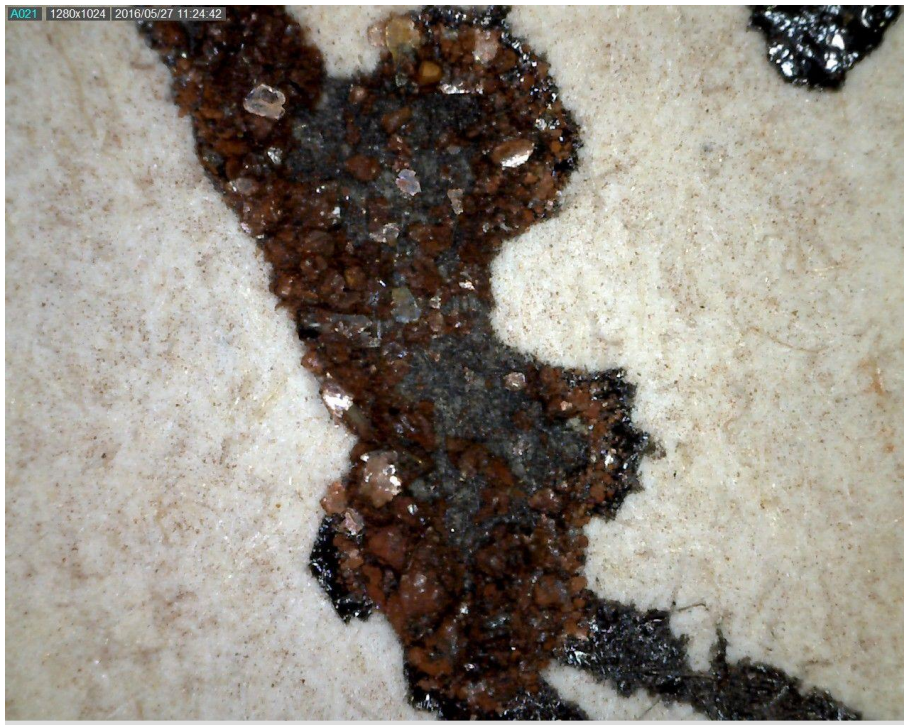
Fig. 18. UBL Or. 6353a, f. 125a. Black ink with particles of quartz sand, coated with iron-oxide © Courtesy UBL.
