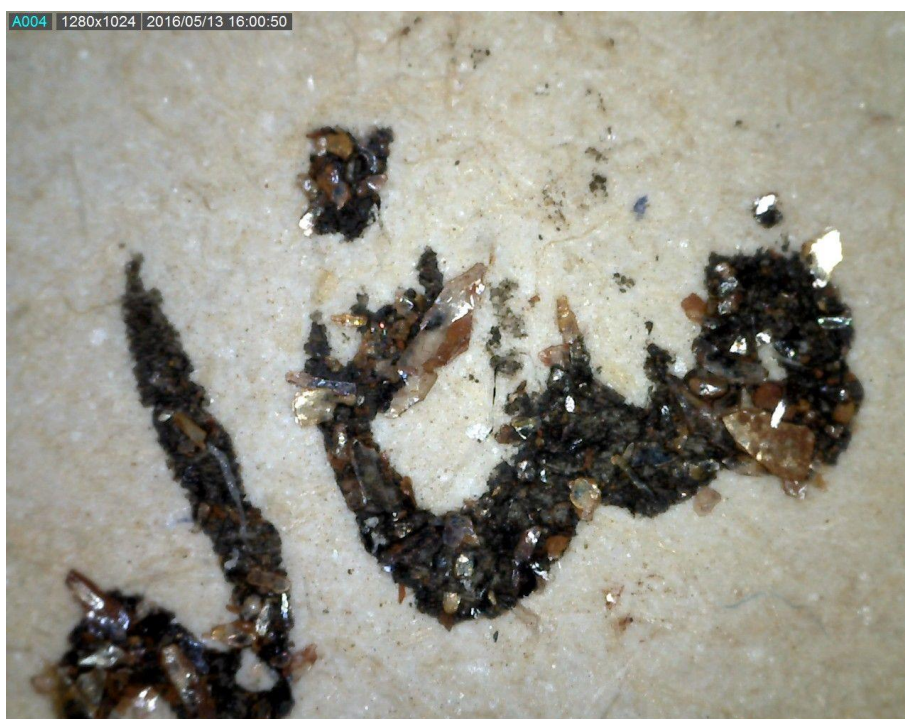
Fig. 16. UBL Or. 6643, f. 37b. Diversity in appearances of mica particles © Courtesy UBL.
