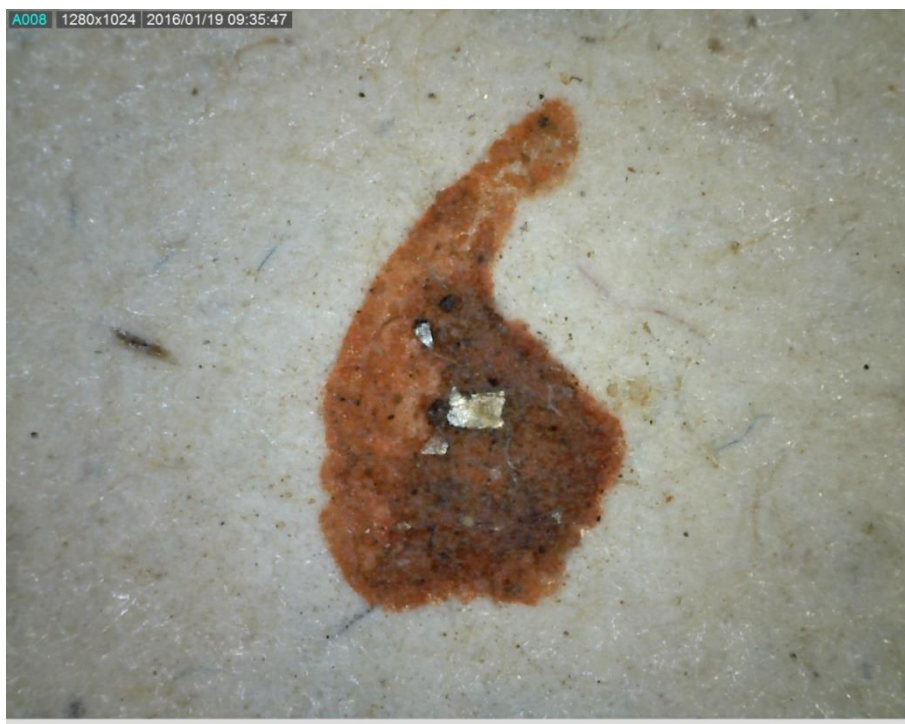
Fig. 12. UBL Or. 2722, f. 4. Red ink containing lead and flake of gold © Courtesy UBL.
