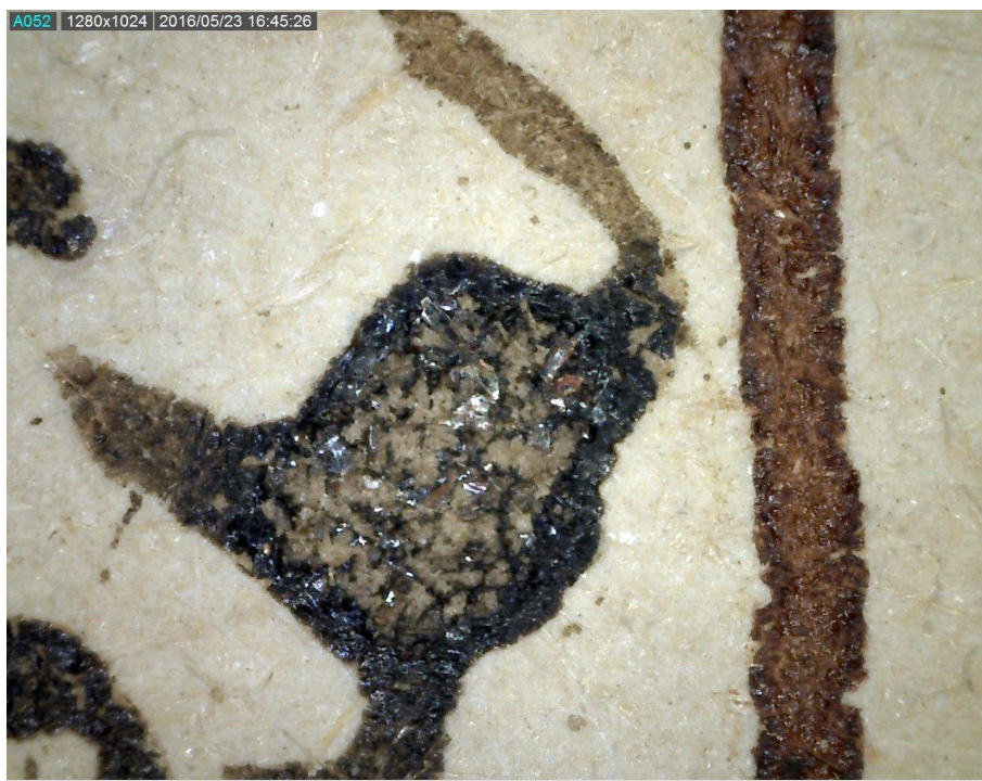
Fig. 20a. UBL Or. 23.448, f.1a. Loss of ink because of the loss of particles © Courtesy UBL.
