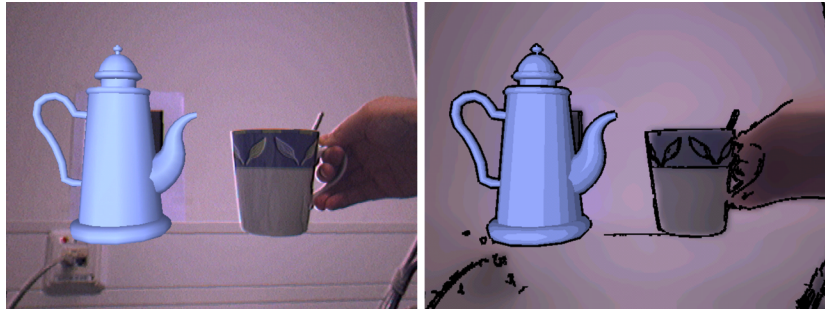
Figure 4.7: A comparison between traditional augmented reality (left) and stylized AR (right) as implemented by Fischer et al. (2005). In both images, the teapot is a virtual object, while the cup and the hand are real. However, the stylized version uses an image filter and non-photorealistic rendering. Reprinted from J. Fischer et al. (2005). “Stylized augmented reality for improved immersion”. In: Proceedings IEEE Virtual Reality 2005 . IEEE, pp. 195–202. Reprinted under fair use.
