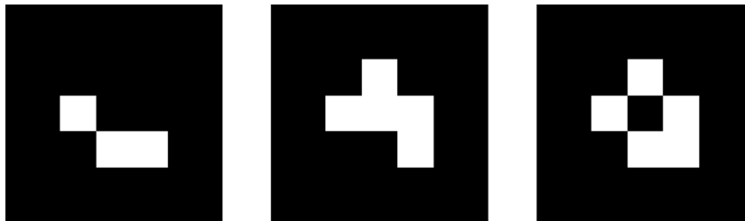
Figure 3.3: Three typical fiducial markers that can be recognized by AR software, such as the popular open-source ARToolkit tracking library. (The displayed markers are part of the download of the ARToolkit SDK (1999).)
