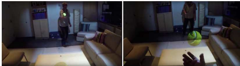
Figure 3.4: The projection-based AR project by Benko et al. (2014) can make it seem as if virtual objects existed in real space, rather than projected onto the world. The image shows two screenshots from the YouTube video about this project (Microsoft Research, 2014).
