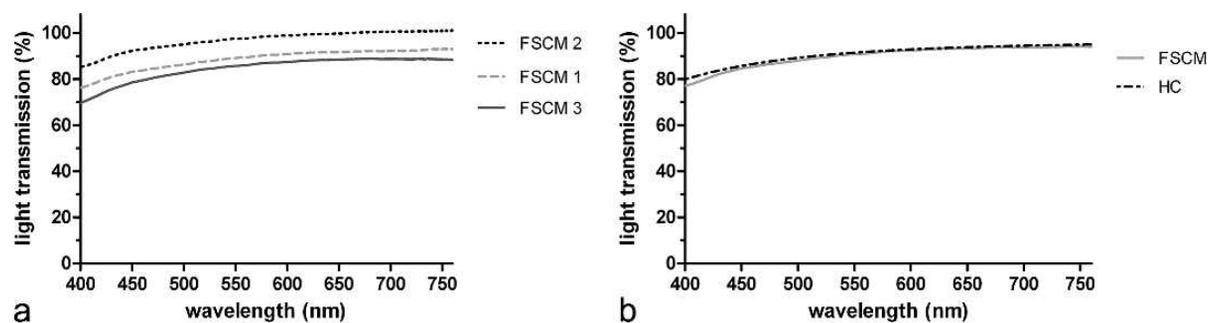
**Figure 4.** Direct light-transmission curves for the visible spectrum of three FSCMs (a), and the mean direct light transmission of the FSCM compared with the total light transmission of the human cornea (b). HC, human cornea.
