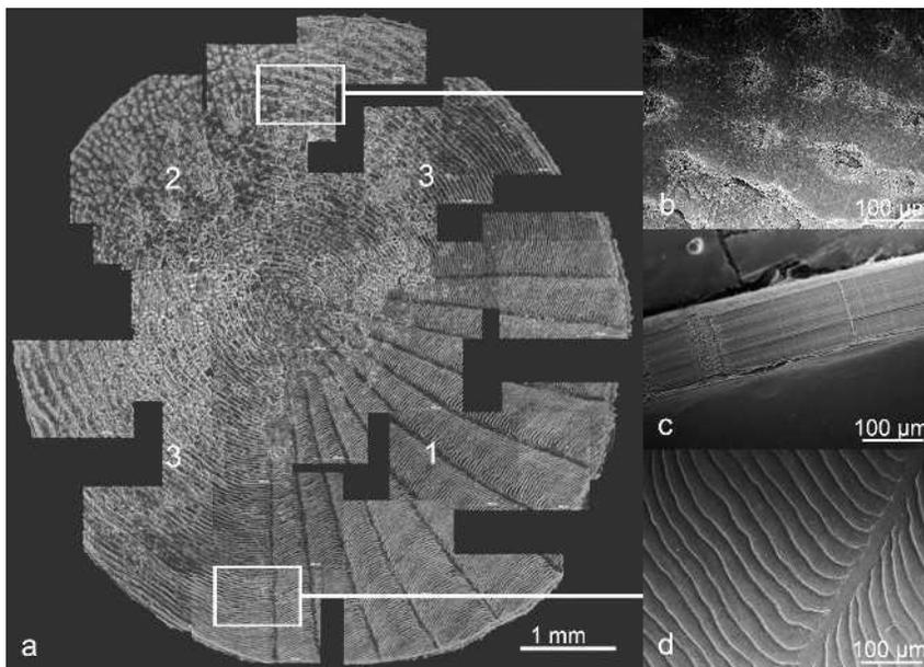
**Figure 2.** Composition of several phase-contrast images showing the distribution of the micro pattern with the spokes and interconnecting channels in one quadrant (a-1), the spikes in the opposite quarter (a-2), and the circular running lines in the area (a-3) between those two quadrants. Detailed SEM-images depict the transitional area between the circular lines and spikes (b), between the lines and spokes (d), and a cross section showing the multiple layers (c).
