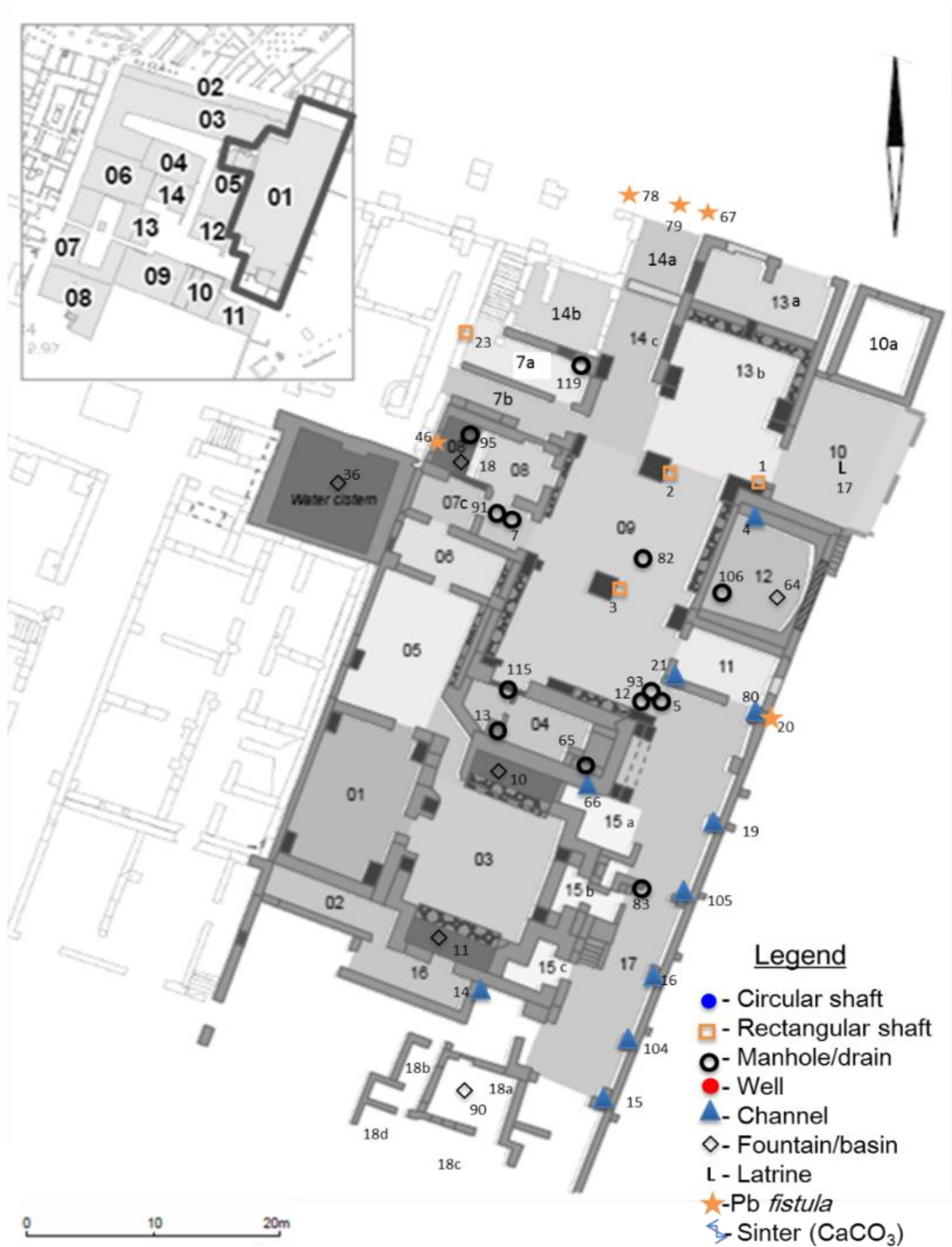
Figure 4.111: Identified water features in the Terme del Faro (after Stöger 2011, 79, Fig. 5.16).
