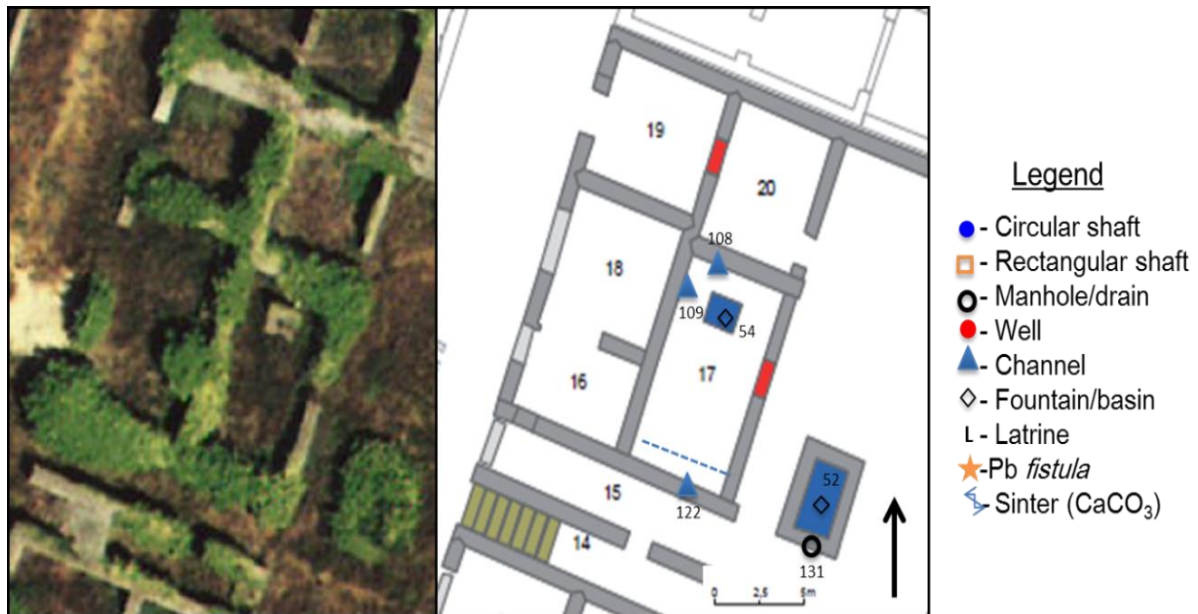
Figure 4.150: View of the northwest corner of IV, ii, 7 from above at left (Mannucci 1995, Pl. 44), and with identified water features on right (Stöger 2011, 124, Fig. 5.68).
