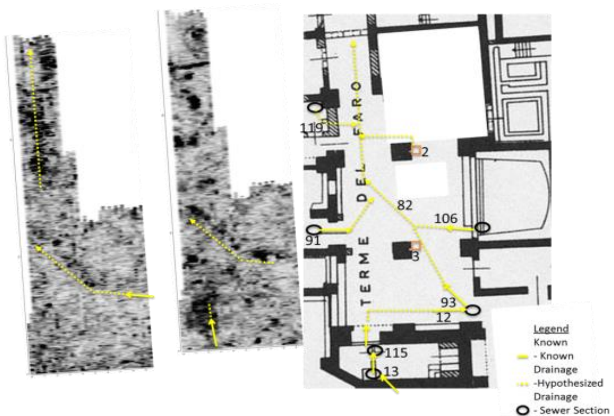
Figure 4.180: Two depth slices of the ground penetrating radar study of the Terme del Faro (IV, ii, 1), with identified and hypothesized sewer features indicated by solid and dashed lines respectively.
