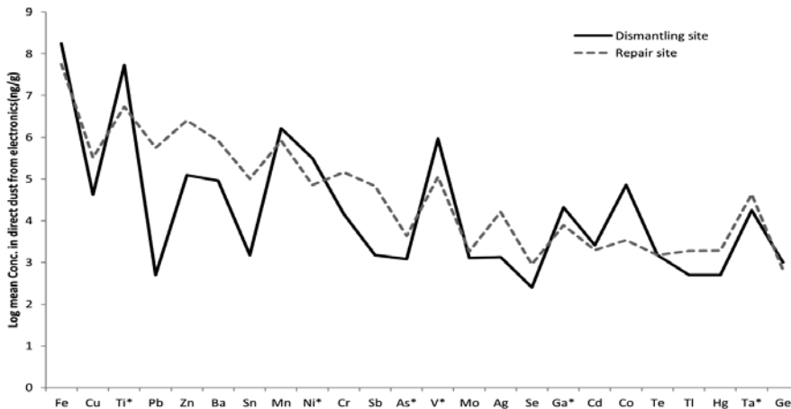
Fig. 4.7. Metal concentrations in direct dust from electronics. Metal concentrations with significant difference are indicated with*.
