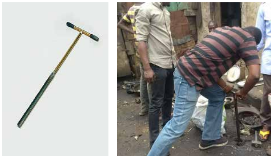
Figure 1.5: Soil Sampling using Dutch Soil Auger (left) at one of the E-waste Recycling Sites Photo credit: Chimere May Ohajinwa, 2015
